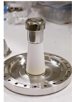
High voltage processing in the presence of inert gas (He and Kr) was demonstrated to significantly improve the performance of stainless steel and niobium cathode electrodes, eliminating field emission ( $< 10\text{ pA}$ ) at voltages to 225 kV and field strengths  $> 18\text{ MV/m}$  [217] (see Fig. 4.6).
