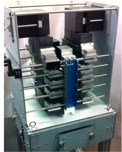
(b) Permanent magnet for beam focusing
