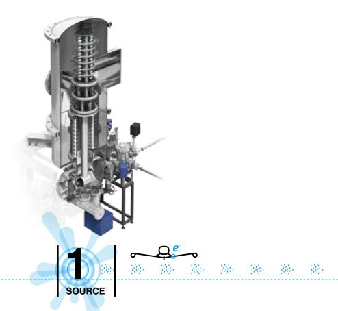
Electrons are produced in the electron source. An intense laser beam shines onto a semiconductor cathode and knocks out billions of electrons.
